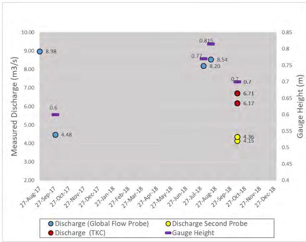
Figure 8 Lower Ibex River gauge height and measured discharge vs date
