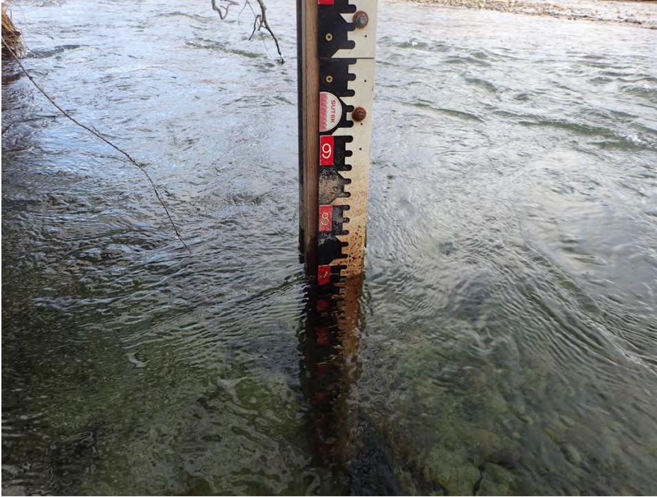
*Figure 5 Water level gauge at lower Ibex River station*
