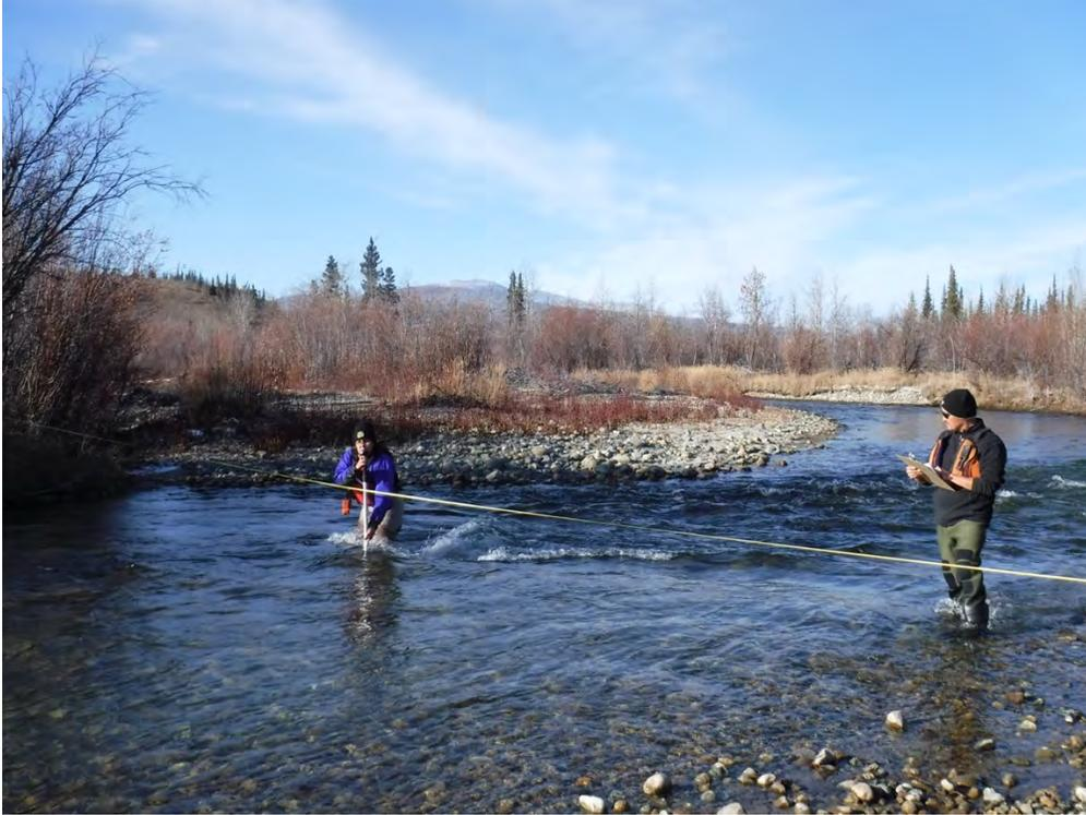
*Figure 6 Cheyenne Bradley, KDFN citizen working on YF&G project, (left) measuring water velocity, and Bruce Wilson, KDFN Land Steward, recording measurements at the Ibex water station site*
