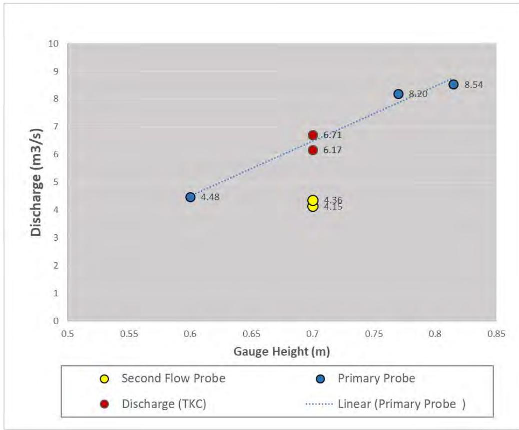
Figure 9 lower Ibex River measured discharge vs. gauge height, 2017-2018
