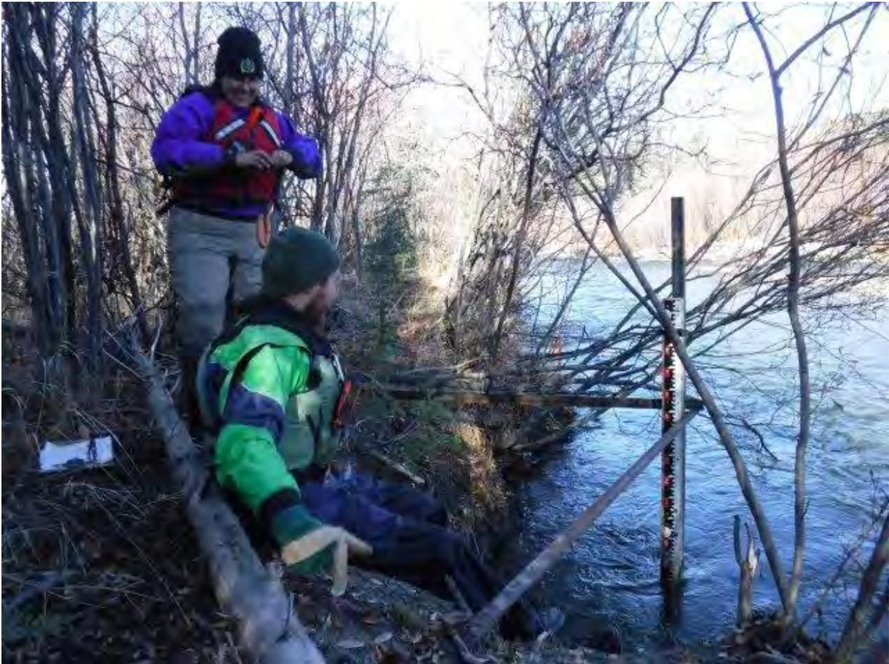
Figure 1 Lower Ibex River Water Level Monitoring Station
